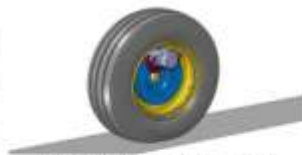
Figure 2: Abaqus tire, road and brake model
