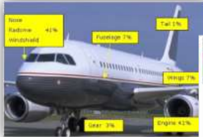
Statistical distribution of impact damage
